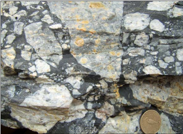
Figure 14: Monomict dacite breccia with dark pyritic matrix (grades ~2g/ton Au), intermediate to a dacite with stockwork-style brecciation and the polymict breccias endmember breccia phases (with breccia clasts of dacite, andesite, basement metamorphic rocks, country rock sediments, etc.) within the hydrothermal breccia body. Photo courtesy of K. Rasmussen.
