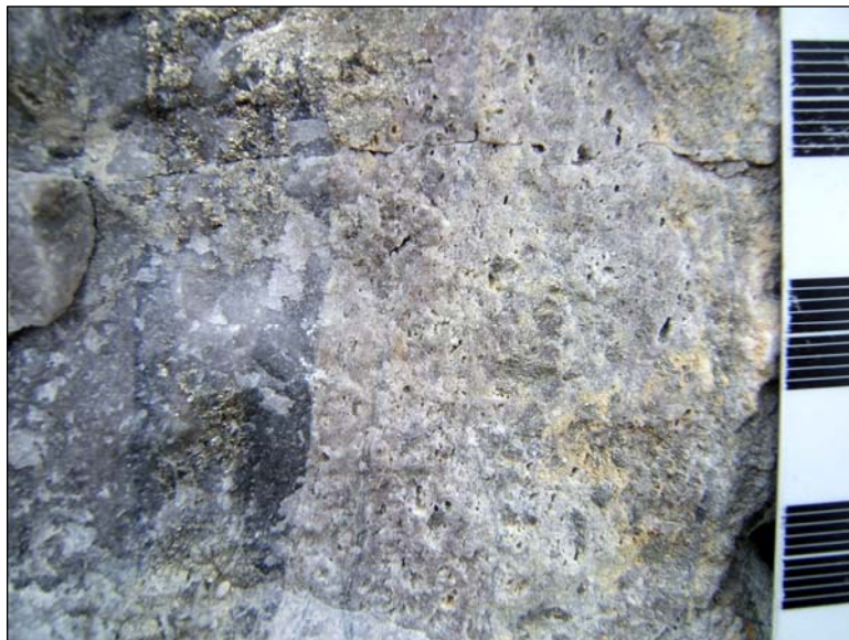
Figure 20: Example of evidence for late-stage, high sulphidation hydrothermal system: steeply dipping quartz-pyrite-enargite veins with vuggy silica alteration (SiO 2 destructive) halos cross-cutting porphyry mineralization. Photo courtesy of K. Rasmussen.
