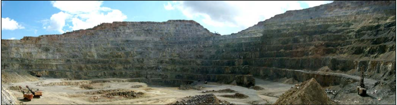
Figure 18: Panorama of the open pit at the Rosia Poieni Cu-Au Mine. Alteration is visible as a red supergene cap, adjacent palest grey advanced argillic alteration, and pale-medium yellowy grey phyllic alteration in gradational contact with darkest grey potassic alteration in the lower pit walls and the pit floor. Photo courtesy of A. Soful.
