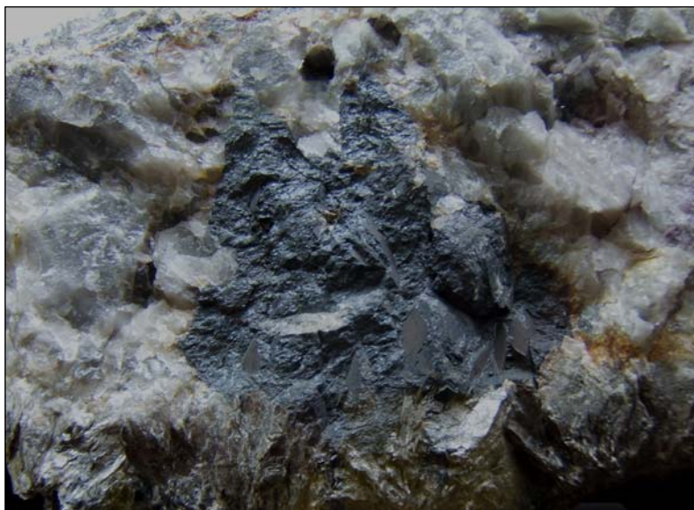
Figure 6: Representative quartz vein with elongate wolframite and stubby cassiterite, and zinnwaldite along vein margin. Sample is 10cm high. Photo courtesy of K. Rasmussen.
