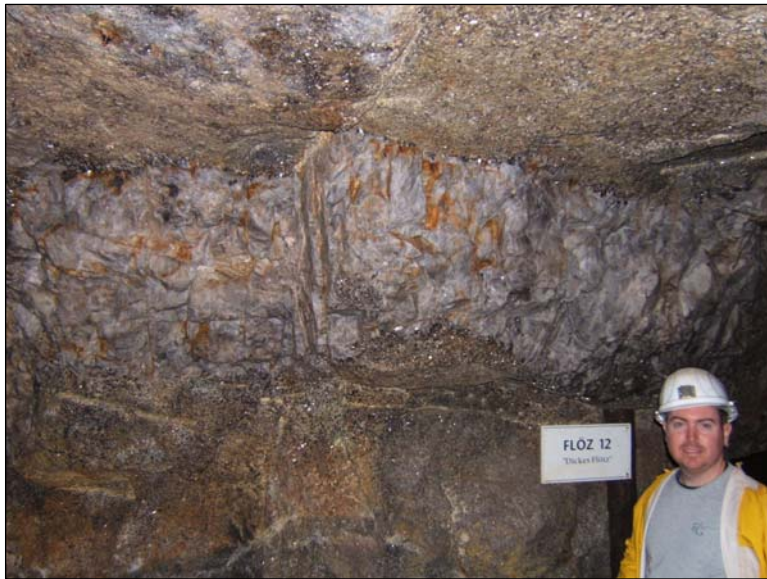
Figure 5: A shallow-dipping, high-grade Sn-W quartz vein with dark, sub-metallic cassiterite and wolframite visible at vein margins and with a wide greisenized halo. Photo courtesy of K. Rasmussen.
