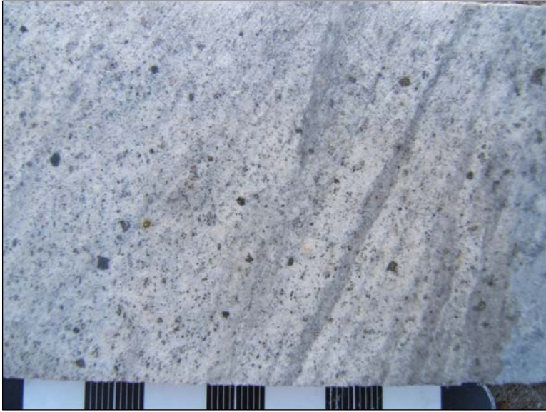
Figure 21: Drill core showcasing high-grade (4.17g/ton Au), banded, argillically altered andesite (with sericite in feldspar) from the East zone, Certej Au-Ag epithermal deposit. Gold mineralization is found within the pyrite cubes. Photo courtesy of K. Rasmussen.
