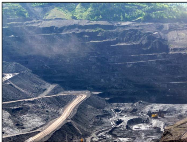
Thrust-stacked, repeating coal seams (visible in the pit wall dipping to the right) has led to localized thickening of coal seams, allowing for profitable open pit mining.
