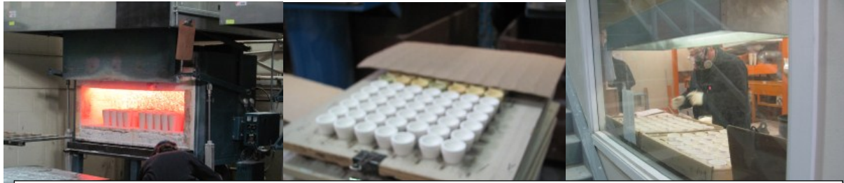
Fire Assay: (Left to Right): crucibles in the furnace, unused cupels, flux station with automated mixer
